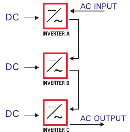
Mains backup with triple redundancy for critical applications
